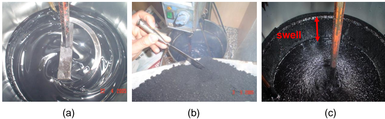
Figure 1 – Continuous blend asphalt rubber produced at laboratory
